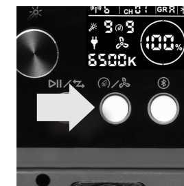
3. Turn the button and then rotating effects dial, you can adjust the frequency of the effect.
